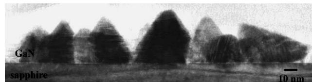
Figure 5. A HREM image of the 120 s nucleation layer.
